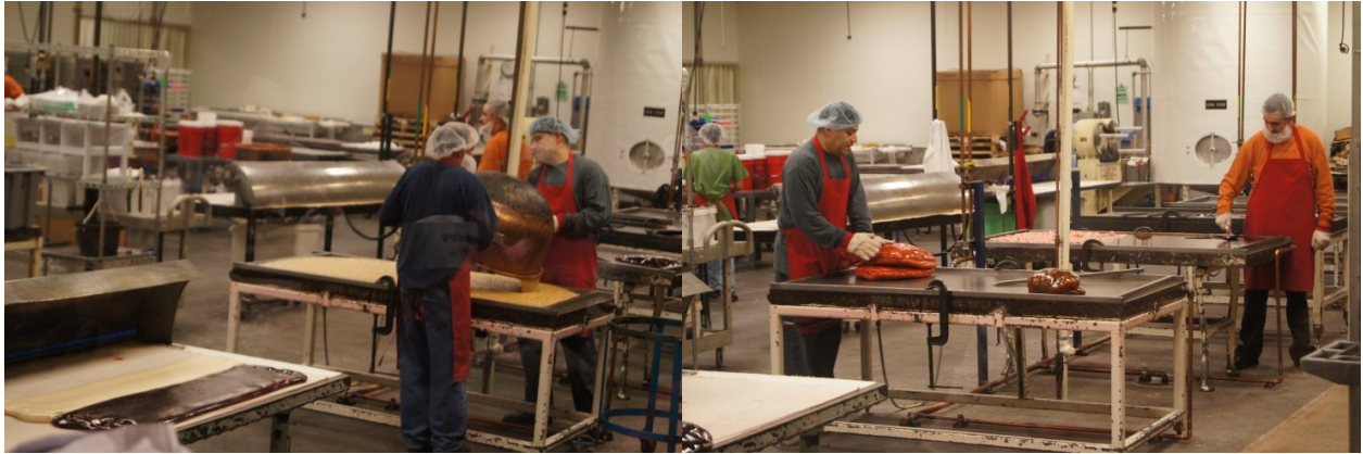
The first photo above shows workers pouring a fresh batch of candy onto a cooling table. A dark red slab of soft candy is on the table at the lower left. A white slab of candy is to its left. The second photo shows the workers folding up candy that has sufficiently cooled.
