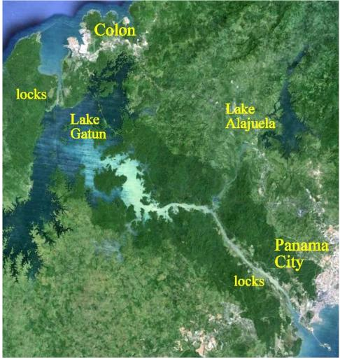
77 km (48 miles) and the Zone width is 16 km (10 miles). The lake and canal water is fresh water from rainfall only. Additional water is provided by Lake Alajuela.
