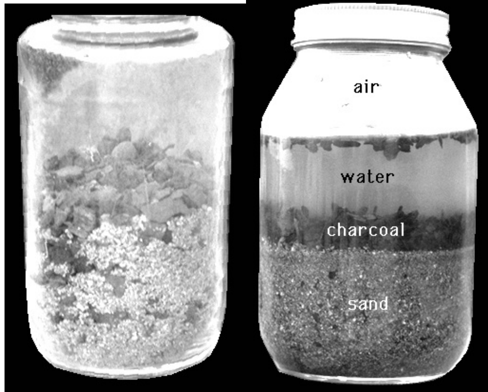
Figure A10-2. If a charcoal and sand mixture is dry or slightly wet, it can remain mixed, as in this jar. Vibrations can cause the sand to sink and the charcoal to rise.
