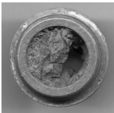
Figure A9-2. Concretion deposits in bathroom pipe.
