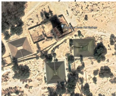
Hot water tower at top, 3 cooling pyramids in this Google Earth view
