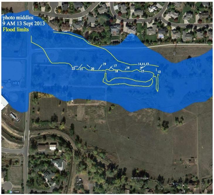
The white lines and numbers mark the approximate middles of photos taken at 9 AM 13 September 2013, after the flooding peak. The water did not cross the roadways except in one location in the middle. The water ran backwards through a culvert between photo locations 17 and 19. The cluster of photos 11-15 are of where the water ran over a pathway and large culvert. Two later photos show the water receding there.
